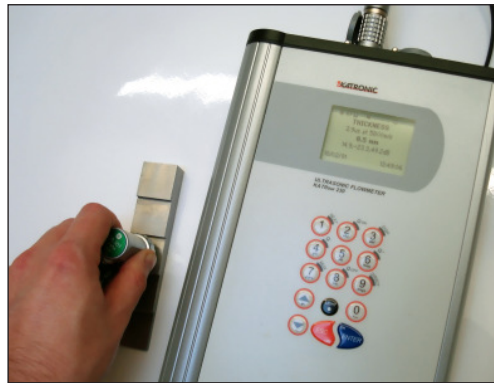
Wall thickness gauge used with KATflow 230
