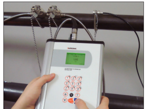
KATflow 230 used as portable heat meter
